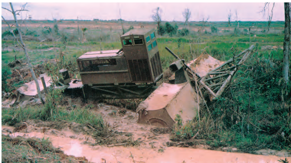
The limitations of the transphibian tactical tree crusher outweighed its benefits, and the equipment was returned to the United States after the lease expired.
